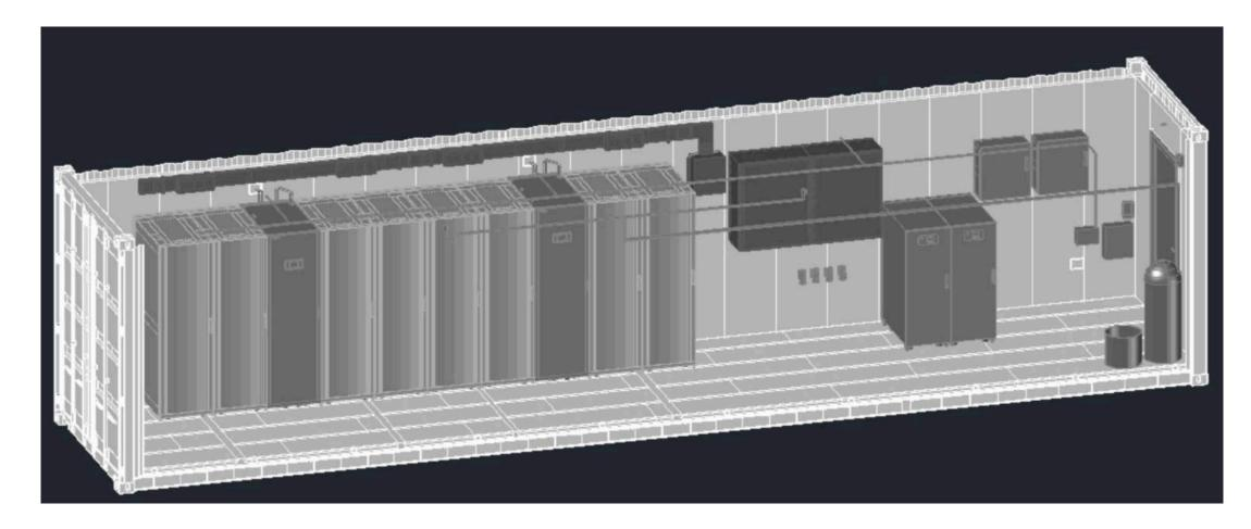
Uniteam Data Center turns a 40 ft High Cube ISO Container into a plug-and-play data-centre. Factory-built and pre-tested, it drops on-site, connects to power and fibre, and is live within hours—no building works, no long lead times. Sliding racks rows make maintenance effortless, while the layout is already prepared for docking extra units as demand grows. The result: fast, low-risk capacity wherever you need it, at a fraction of the usual investment.
