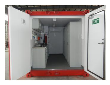
Uniteam Offshore Workshop is designed, manufactured and certified in accordance with DNV 2.7-1/EN 12079 and also DNV 2.7-2 if required. The units can be supplied in various sizes with certified slings and shackles, as well as, cabinets, pull-out shelves and other equipment, according to customer's needs. It is designed for repairs, maintenance, storage of equipment and tools, providing you a safe and comfortable work environment for the oil & gas industry.
