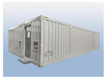
Uniteam 30men H2S shelter (SIP) is a highly customized solution built for easy transport and relocation at Malaysia offshore platform. It is made up of 4 sets of containers (2x40', 1x20' and 1x10'), has an A-60 fire rating. The sealing between the containers is solved by Uniteam patented GSSP gaskets which ensuring quick deployment of SIP on-site with minimal downtime to the ongoing production. Moreover, all equipment is IECEX certified and can be used in Zone 1 or Zone 2 hazard area.
