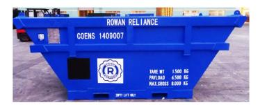
Uniteam Offshore Waste Skip are designed, manufactured and certified in accordance with DNVGL 2.7-1, as well as EN 12079. An open or closed offshore skip are used for the storage and removal of waste. Normally constructed from flat steel plates forming the load bearing sections of the container, bracing in the form of steel profiles, e.g. channel or hollow section, being fitted horizontally around sides and ends. Waste skips may be open or have loose or hinged covers.
