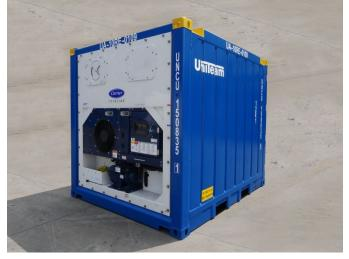
Uniteam Offshore Reefer Containers are designed, manufactured and certified in accordance with DNV 2.7-1, as well as EN 12079 and IMO/MSC Circular 860. It is suitable for storing and transporting frozen and chilled food. The container is equipped with CARRIER, THERMO KING or DAIKIN refrigeration unit to maintain the indoor temperature between -25  $^\circ$  and +25  $^\circ$ .
