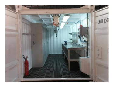
Uniteam Offshore Workshop with Crane is designed, manufactured and certified in accordance with DNV 2.7-1/EN12079. It can also be delivered according to DNV 2.7-2 if required. This unit is designed for repairs, maintenance, storage of equipment and tools, providing you a safe and comfortable work environment for the oil & gas industry. The crane allowed for easy movement of equipment and can be supplied according to your requirements.
