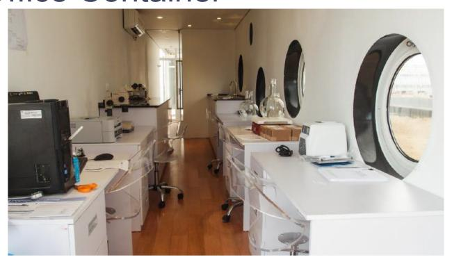
Uniteam Offshore Office Container are designed, manufactured and certified in accordance with DNVGL 2.7-1, as well as EN 12079. The units can be supplied in various sizes with certified slings and shackles, as well as, decoration, floor, window, lighting design, workbench and other equipment, according to customer's needs. The end have a washroom with a chemical toilet .
