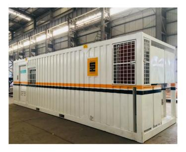
Uniteam Offshore Mud Logging in China are built according to DNV.GL 2.7-1 / DNV GL 2.7-2 / IEC60079-13, The cabin with A60 fire rated decoration and EX approved for use in Zone 1 / Zone 2 area. Pressurized cabin with HVAC system. The cabin included air lock, main room, and equipment room.
