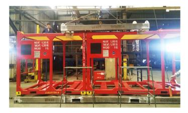
Uniteam Offshore pump skids are designed, manufactured and certified in accordance with DNV 2.7-1 and DNV 2.7-3, as well as EN 12079. These skids are designed for transport pumps to platform. 2 units of skids fixing on base skid, It can be easily installed and removed fast from base skid. It has specialized spreader frame to sling the modules. The advantage is that can move easily and fast when maintaining pumps or generator.
