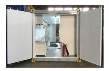
Uniteam Offshore Mud Lab Container is designed, manufactured and certified in accordance with DNV 2.7-1/EN 12079 standard. The module is composed of container body, fume hood cabinet, workbench, storage cabinet, air condition, transformer, water heater, refrigerator and so on. The equipment satisfy customer's needs. It is designed for mud lab drilling, providing a safe and comfortable work environment for the oil & gas industry.
