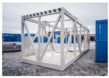
The attached DNV 2.7-3 Oversized Lifting Frame was designed for transportation of wide range of cargo included ISO containers and other onshore units within offshore conditions. Frame is equipped in 42 pcs. of lashing rings to secure cargo and secured from the slings snugging by a special tarpaulin.
